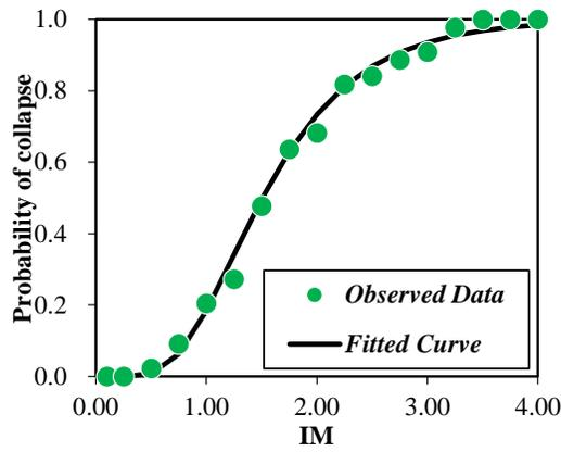
Figure 5. Sample Fragility Function Curve Fitting
