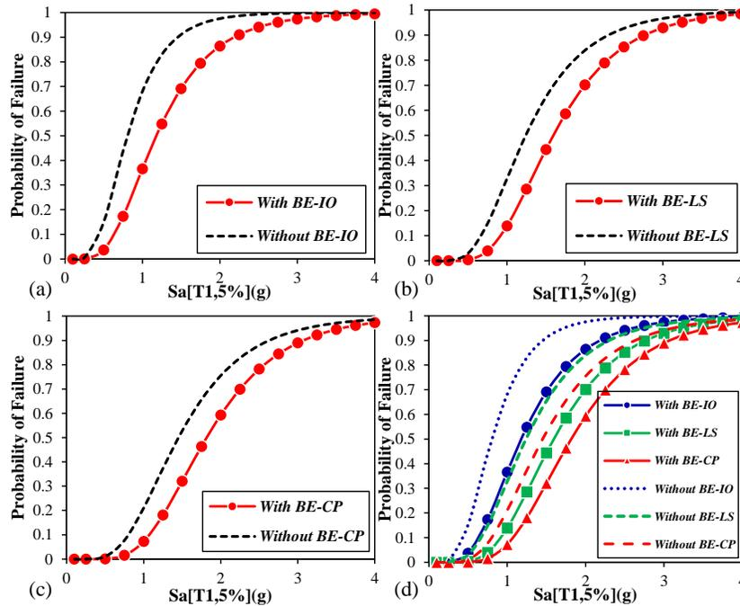
Figure 6. Fragility Curves of different Performance Levels: (a) IO; (b) LS; (c) CP; (d) Comparison of different performance levels
