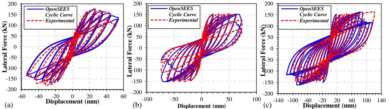
Figure 2. Comparison of Numerical versus Experimental Hysteretic loops: (a) W1; (b) W2; and (c) W3 (Experimental data from Shedid et al. 2010)
