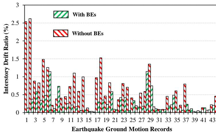
Figure 8. Inter-Story Drift Variation of the RMSW Building before and after having Boundary Elements
