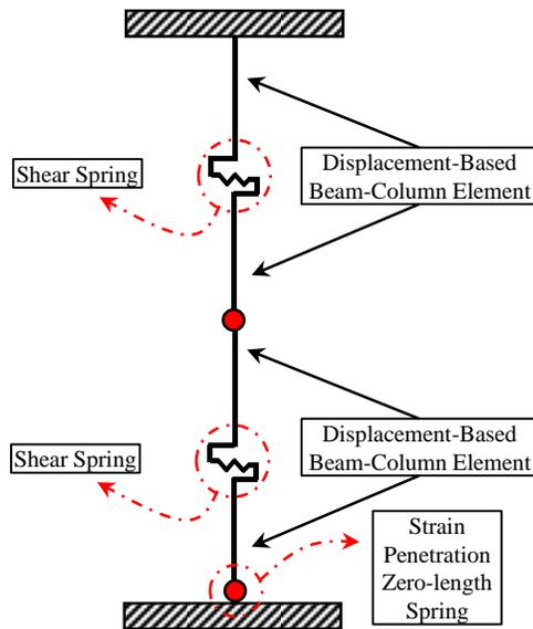
Figure 1. Schematic element assembly of the shear wall segment
