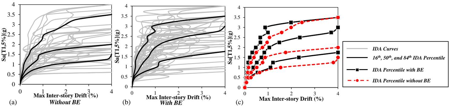
Figure 4. IDA Curves and 16th, 50th, and 84th percentile: (a) RMSW Building without Boundary Element; (b) RMSW Building with Boundary Element; (c) Comparison of the results.
