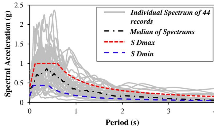
Figure 3 Response Spectrum of 44 unscaled Ground motions along median spectrum; Upper bound ( $S_{Dmax}$ ); and Lower bound ( $S_{Dmin}$ )
